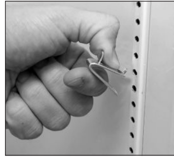
Fig. 1. Installing top tab of shelf clip.
