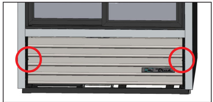
Fig. 2. Slide door louver grill screw locations.
