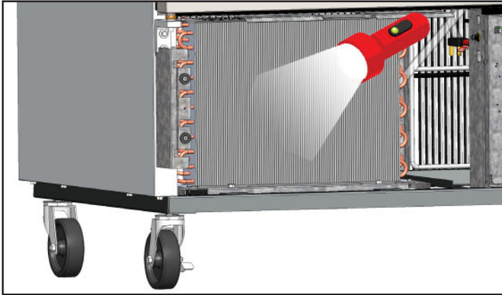
Fig. 5. Verify all blockages have been removed.
