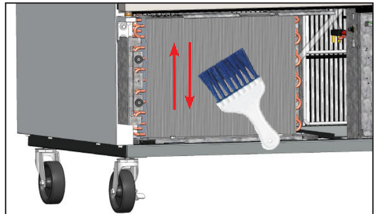
Fig. 4. Never brush across the coil fins.
